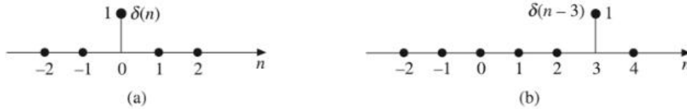
Figure 1.9 Discrete-time (a) Unit sample sequence, (b) Delayed unit sample sequence.
