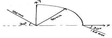
b) Find the Centroid for the shaded area about y – axis. As shown in the Figure
