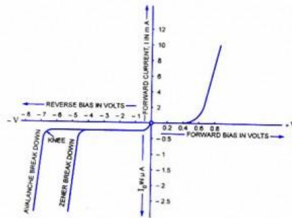
Fig 1.18: Diode characteristics with breakdown
