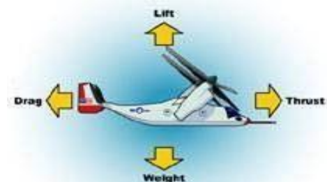
Fig: Four Forces on an Airplane (Ref: NASA)
