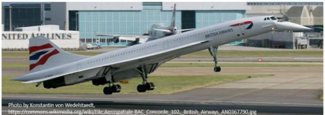
Concorde just prior to touchdown with forward nose rotated downward
