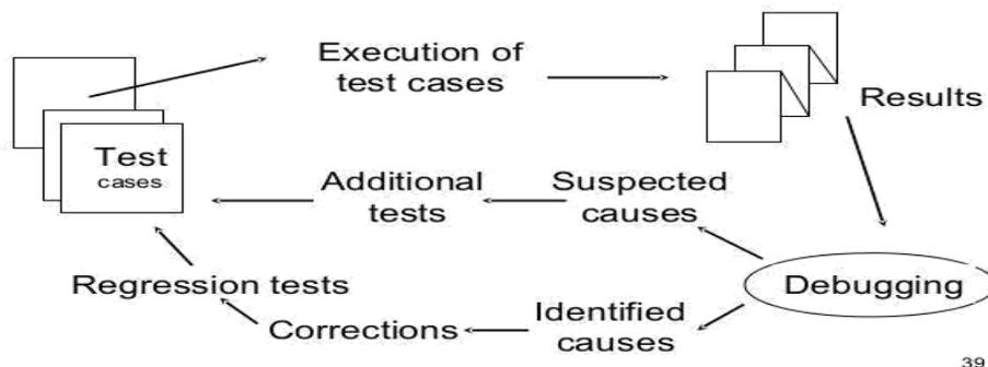
Fig: Debugging process
