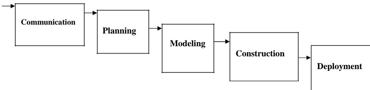
This Model suggests a systematic, sequential approach to SW development that begins at the system level and progresses through analysis, design, code and testing
