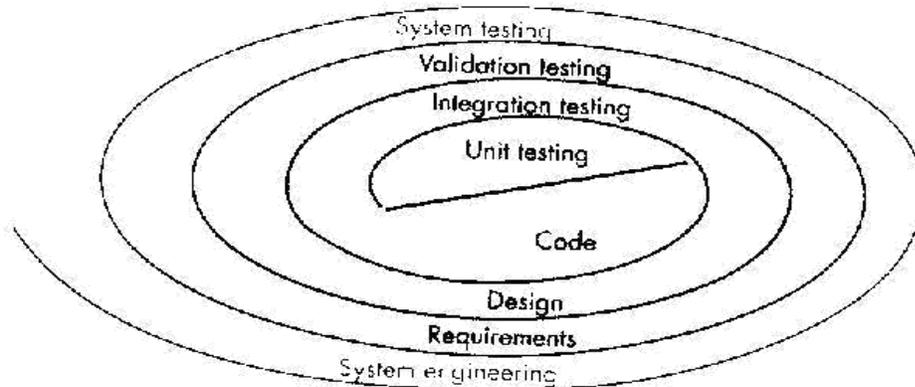
**Unit Testing** begins at the vortex of the spiral and concentrates on each unit of software in source code.
