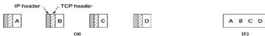
Figure 4-13. (a) Four 512-byte segments sent as separate IP datagrams. (b) The 2048 bytes of data delivered to the application in a single READ call.
