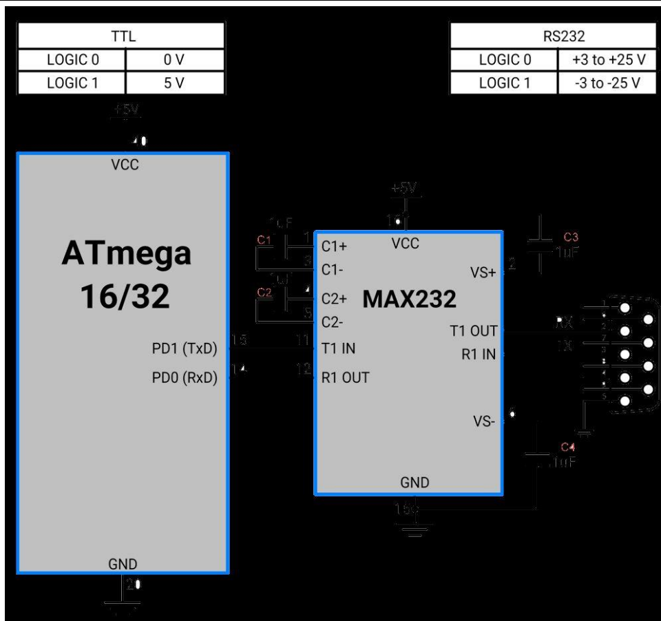
ATmega16/32 Serial Interface Connection Diagram
