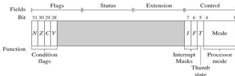
FIGURE 2.4 Format of the program status registers.
