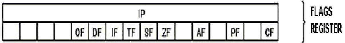
Flag Registers Intel 8086-8088 Microprocessor
