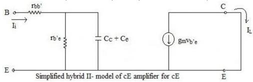
$$A_i = \frac{I_C}{I_i} = \frac{-g_m I_i}{\frac{1}{r_{b/e}} + j\omega(C_C + C_e)}$$
