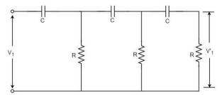
Each section produces a phase shift of  $60^{\circ}$ . Consequently, a total phase shift of  $180^{\circ}$  is produced, i.e., voltage  $V_2$  leads the voltage  $V_1$  by  $180^{\circ}$ .
