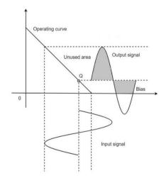
The small bias voltage given using diodes  $D_1$  and  $D_2$ , as shown in the above figure, helps the operating point to be above the cutoff point. Hence the output waveform of class AB results as seen in the above figure. The crossover distortion created by class B is overcome by this class AB, as well the inefficiencies of class A and B don't affect the circuit.
