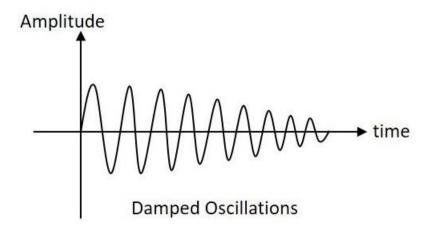
Damped oscillations are generally produced by the oscillatory circuits that produce power losses and doesn't compensate if required.
