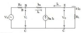
$$A_{I} = \frac{I_{0}}{I_{b}} = \frac{-I_{e}}{I_{b}} = \neq \neq \frac{(1 + h_{fe})J_{b'}}{I_{b'}} = 1 + h_{fe}$$
