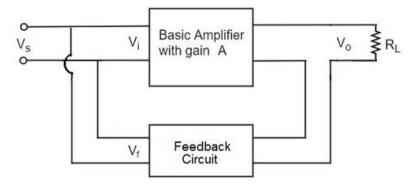
As the feedback circuit is connected in series with the output, the output impedance is increased and due to the parallel connection with the input, the input impedance is decreased.
