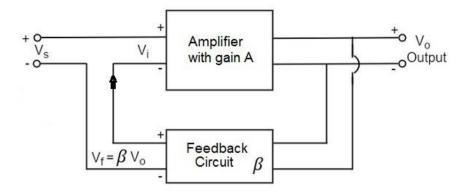
From the above figure, the gain of the amplifier is represented as A. The gain of the amplifier is the ratio of output voltage Vo to the input voltage  $V_i$ . The feedback network extracts a voltage  $V_f = \beta V_o$  from the output  $V_o$  of the amplifier.
