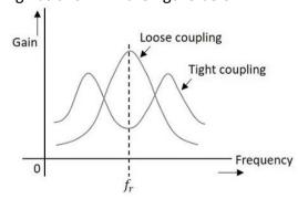
On the contrary, when the primary and secondary coils are brought close together, they have **Tight coupling**. Under such conditions, the reflected resistance will be large and the circuit Q is lower. Two positions of gain maxima, one above and the other below the resonant frequency are obtained.
