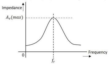
At resonant frequency  $f_r$  the impedance of parallel tuned circuit is very high and is purely resistive. The voltage across  $R_L$  is therefore maximum, when the circuit is tuned to resonant frequency. Hence the voltage gain is maximum at resonant frequency and drops off above and below it. The higher the Q, the narrower will the curve be.
