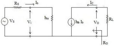
$$A_{I} = \frac{I_{0}}{I_{h}} - \frac{h_{fe} I_{h}}{I_{h}} = -h_{fe}$$
