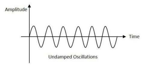
Undamped oscillations are generally produced by the oscillatory circuits that produce no power losses and follow compensation techniques if any power losses occur.
