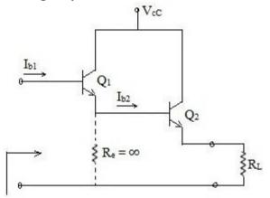
Darlington pair 1- Two emitter follower stages in cascade with infinite emitter resistance in the first stage constitute a Darlington circuit.
