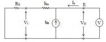
$$\therefore \quad R_o = \frac{h_{ie} + R_S}{1 + h_{fe}}$$
