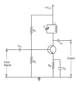
The output can be obtained from the coupling capacitor  $C_{\mathbb{C}}$  as shown above or from a secondary winding placed at L.
