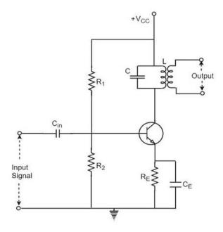
The tuner circuit is nothing but a LC circuit which is also called as **resonant** or **tank circuit**. It selects the frequency. A tuned circuit is capable of amplifying a signal over a narrow band of frequencies that are centered at resonant frequency.
