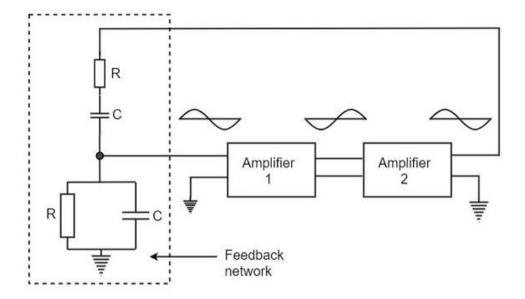
The oscillator consists of two stages of RC coupled amplifier and a feedback network. The voltage across the parallel combination of R and C is fed to the input of amplifier 1. The net phase shift through the two amplifiers is zero.
