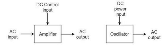
The frequency, waveform, and magnitude of a.c. power generated by an amplifier, is controlled by the a.c. signal voltage applied at the input, whereas those for an oscillator are controlled by the components in the circuit itself, which means no external controlling voltage is required.
