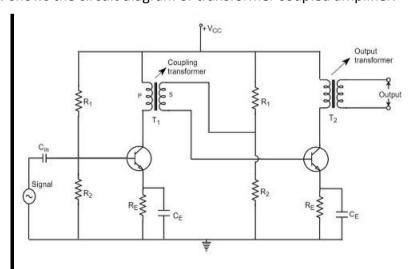
The potential divider network  $R_1$  and  $R_2$  and the resistor  $R_e$  together form the biasing and stabilization network. The emitter by-pass capacitor  $C_e$  offers a low reactance path to the signal. The resistor  $R_L$  is used as a load impedance. The input capacitor  $C_{in}$  present at the initial stage of the amplifier couples AC signal to the base of the transistor. The capacitor
