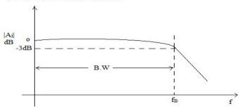
The parameter  $f_T$ : The frequency at which the magnitude short ckt. current gain of  $C_E$  amplifier reduces to unity is
