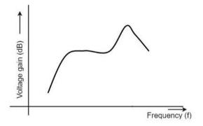
At low frequencies, the reactance of primary begins to fall, resulting in decreased gain. At high frequencies, the capacitance between turns of windings acts as a bypass condenser to reduce the output voltage and hence gain.
