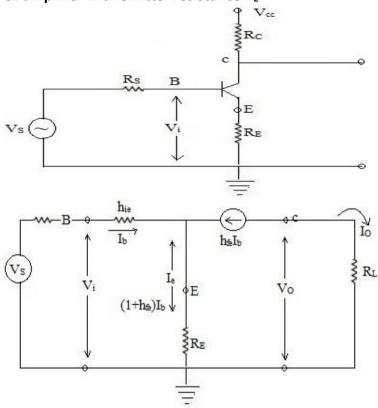
$$A_{\rm I} = \frac{I_{0}}{I_{b}} = \frac{-h_{\rm fe}I_{b'}}{I_{b'}} = -h_{\rm fe} - - - - - (1)$$
