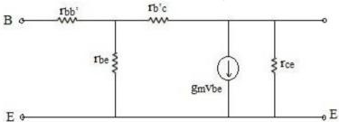
The High frequency model parameters of a BJT in terms of low frequency hybrid parameters is given below
