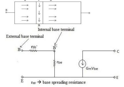
Because the base (B) is lightly doped all the depletion region lies entirely in the Base region. So, when the collector.
