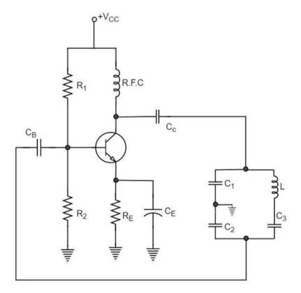
The operation of Clapp oscillator circuit is in the same way as that of Colpitts oscillator. The frequency of oscillator is given by the relation,
