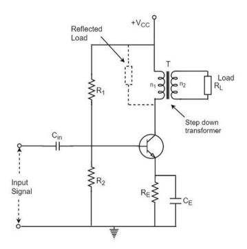
Here  $R_1$  and  $R_2$  provide potential divider arrangement. The resistor Re provides stabilization,  $C_e$  is the bypass capacitor and  $R_e$  to prevent a.c. voltage. The transformer used here is a step-down transformer. The high impedance primary of the transformer is connected to the high impedance collector circuit. The low impedance secondary is connected to the load (generally loud speaker).
