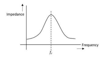
Impedance of the circuit decreases for the values above and below the resonant frequency  $\mathbf{f}_r$ . Hence the selection of a particular frequency and rejection of other frequencies is possible.
