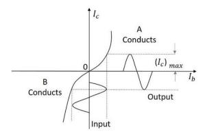
For the next half cycle, the transistor  $T_1$  gets into cut off condition and the transistor  $T_2$  gets into conduction, to contribute the output. Hence for both the cycles, each transistor conducts alternately. The output transformer  $T_{r3}$  serves to join the two currents producing an almost undistorted output waveform.
