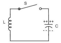
When the switch **S** is closed, the capacitor discharges and the current flows through the inductor. Due to the inductive effect, the current builds up slowly towards a maximum value. Once the capacitor discharges completely, the magnetic field around the coil is maximum.
