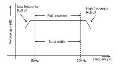
From the above graph, it is understood that the frequency rolls off or decreases for the frequencies below 50Hz and for the frequencies above 20 KHz. whereas the voltage gain for the range of frequencies between 50Hz and 20 KHz is constant.
