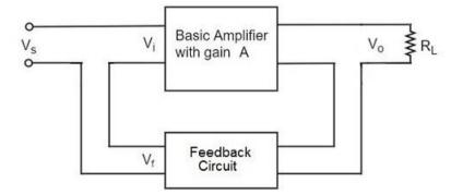
As the feedback circuit is connected in series with the output and the input as well, both the output impedance and the input impedance are increased.
