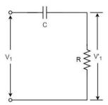
The output voltage  $V_1$ ' across the resistor R leads the input voltage applied input  $V_1$  by some phase angle  $\phi^\circ$ . If R were reduced to zero,  $V_1$ ' will lead the  $V_1$  by  $90^\circ$  i.e.,  $\phi^\circ = 90^\circ$ .
