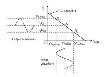
The operating point of this amplifier is present in the linear region. It is so selected that the current flows for the entire ac input cycle. The below figure explains the selection of operating point.
