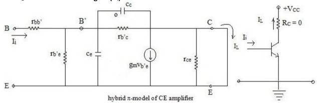
$$\label{eq:gm} g_m = \frac{|I_C|}{V_T}, \qquad r_{b'e} = \frac{h_{fe}}{g_m}, \quad r_{b'c} = \frac{r_{b'e}}{h_{re}}$$
