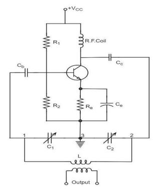
The resistors  $R_1$ ,  $R_2$  and  $R_e$  provide necessary bias condition for the circuit. The capacitor  $C_e$  provides a.c. ground thereby providing any signal degeneration. This also provides temperature stabilization.
