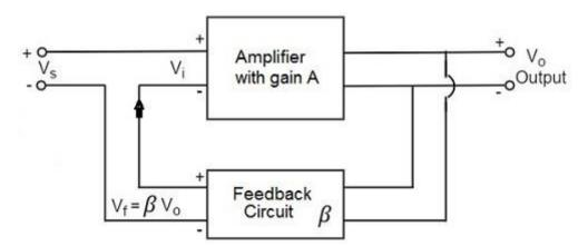
From the above figure, the gain of the amplifier is represented as A. the gain of the amplifier is the ratio of output voltage  $V_0$  to the input voltage  $V_i$ . the feedback network extracts a voltage  $V_f = \beta V_0$  from the output  $V_0$  of the amplifier.
