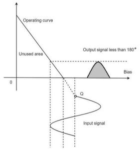
This kind of biasing gives a much improved efficiency of around 80% to the amplifier, but introduces heavy distortion in the output signal. Using the class C amplifier, the pulses produced at its output can be converted to complete sine wave of a particular frequency by using LC circuits in its collector circuit.
