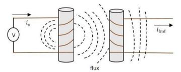
The current  $i_s$  in the figure indicate the source current while  $i_{ind}$  indicates the induced current. The flux represents the magnetic flux created around the coil. This spreads to the secondary coil also. With the application of voltage, the current  $i_s$  flows and flux gets created. When the current is varies the flux gets varied, producing  $i_{ind}$  in the secondary coil, due to the Mutual inductance property.
