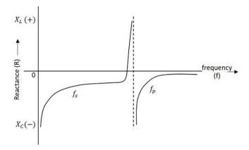
The first one is the series resonant frequency ( $f_s$ ), which occurs when reactance of the inductance (L) is equal to the reactance of the capacitance C. In that case, the impedance of the equivalent circuit is equal to the resistance R and the frequency of oscillation is given by the relation,
