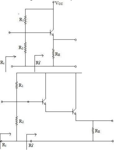
Effective input resistance  $R_i = R_1 \mid R_2 \mid R_i'$  where  $R_i'$  is a large input resistance of emitter follower or Darlington ckt.
