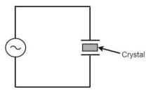
If an AC voltage is applied, the crystal starts vibrating at the frequency of the applied voltage. However, if the frequency of the applied voltage is made equal to the natural frequency of the crystal, **resonance** takes place and crystal vibrations reach a maximum value. This natural frequency is almost constant.
