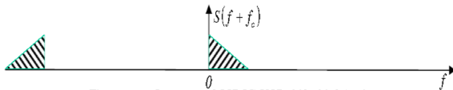
Figure 12 : Spectrum of SSBSC-USB shifted left by f_c
