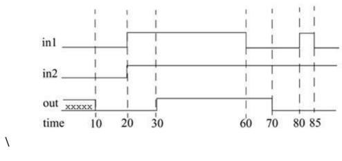
assign #10 out = in1 & in2; // Delay in a continuous assign
