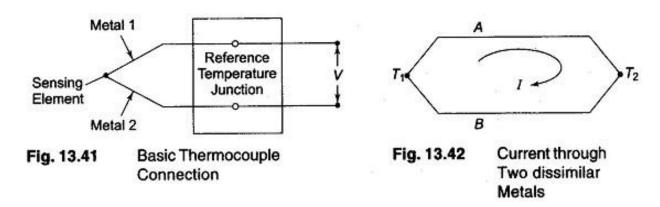
A current will circulate around a loop made up of two dissimilar metals when the two junctions are at different temperatures. When this circuit is opened, a voltage appears that is proportional to the observed seeback current. The Thomson and Peltier emfs originate from the fact that, within conductors, the density of free charge carriers (electrons and holes) increases with temperature.
