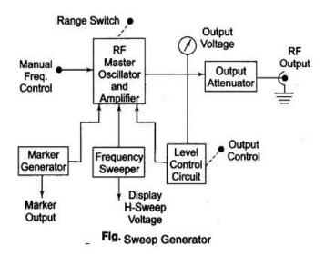
The frequency sweeper provides a variable modulating voltage which causes the capacitance of the master oscillator to vary. A representative sweep rate could be of the order of 20 sweeps/second. A manual control allows independent adjustment of the oscillator resonant frequency. The frequency sweeper provides a varying sweep voltage synchronization to drive the horizontal deflection plates of the CRO. Thus the amplitude of the response of a test device will be locked and displayed on the screen.
