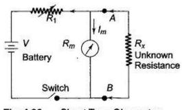
Fig. 4.30 Shunt Type Ohmmeter
