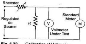
Fig. 4.32 Calibration of Voltmeter
