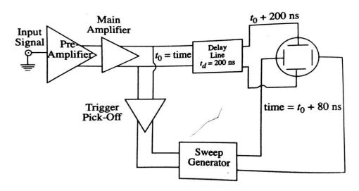
The diagram shows that when the delay line is not used, the initial part of the signal is lost and only part of the signal is displayed. To counteract this disadvantage the signal is not applied directly to the vertical plates but is passed through a delay line circuit.
