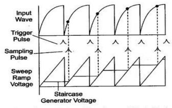
Fig. 7.25 Various Waveforms at Each Block of a Sampling Oscilloscope
