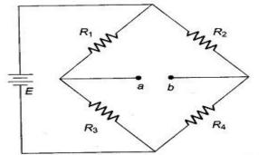
Fig. 11.2 Unbalanced Wheatstone's Bridge
