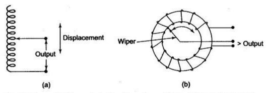
Fig. 13.14 (a) Linear Inductive Transducer (Using Air Core) (b) Angular Inductive Transducer (Using Ferrite Core)
