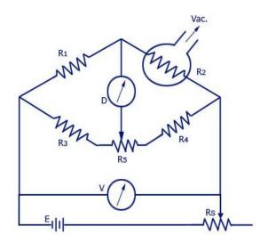
When the pressure changes, there will be a change in current. For this, the voltage V has to be kept constant. The resistance R2 of the gauge is measured, by keeping the gauge current constant. The null balance of the bridge circuit is maintained by adjusting the voltage or current. This change is made with the help of a potentiometer and the change brought will be a measure of the pressure produced.
