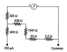
Fig. 4.34 Micro Ammeter Section of a Multimeter
