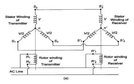
(a) Torque Transmission Using Synchro Trans
