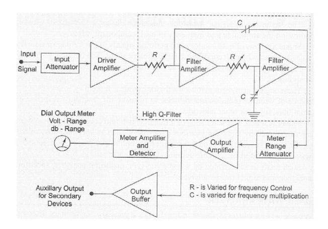
Fig 1: Frequency wave analyzer
