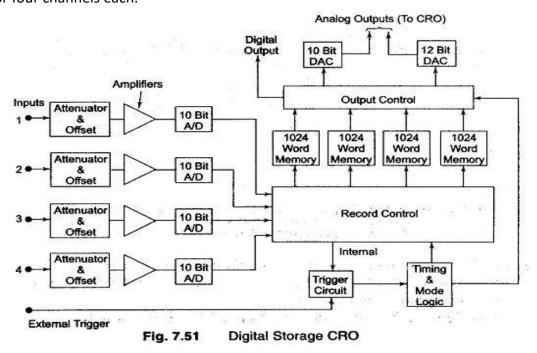
The analog input voltage is sampled at adjustable rates (up to 100,000 samples per second) and data points are read onto the memory. A maximum of 4096 points are storable in this particular instrument. (Sampling rate and memory size is selected to suit the duration and waveform of the physical event being recorded.)
