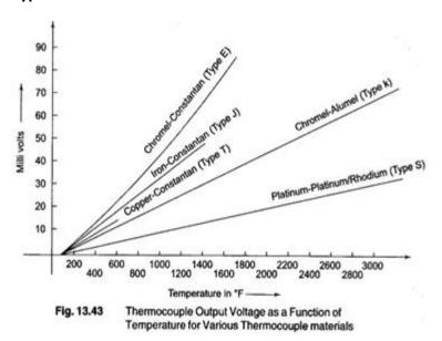
The thermocouple (TC) is a temperature transducer that develops an emf that is a function of the temperature difference between its hot and cold junctions.
