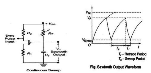
It is necessary that horizontal deflection starts at the same point of the input vertical signal, each time it sweeps. Hence to synchronize horizontal deflection with vertical deflection a synchronizing or triggering circuit is used. It converts the incoming signal into the triggering pulses, which are used for the synchronization.
