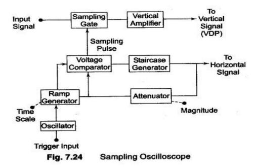
Figure 7.24 shows a block diagram of a sampling oscilloscope. The input waveform is applied to the sampling gate. The input waveform is sampled whenever a sampling pulse opens the sampling gate. The sampling must be synchronized with the input signal frequency. The signal is delayed in the vertical amplifier, allowing the horizontal sweep to be initiated by the input signal. The waveforms are shown in Fig. 7.25.
