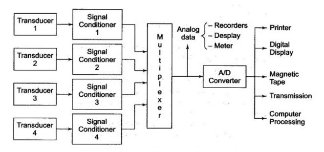
A typical Data Acquisition System consists of individual sensors with the necessary signal conditioning, data conversion, data processing, multiplexing, data handling and associated transmission, storage and display systems.
