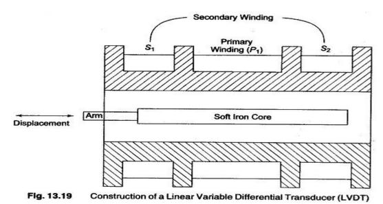
The transformer consists of a single primary winding  $P_1$  and two secondary windings  $S_1$  and  $S_2$  wound on a hollow cylindrical former. The secondary windings have an equal number of
