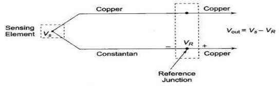
Fig. 13.44 A Type T Thermocouple with Reference Junction
