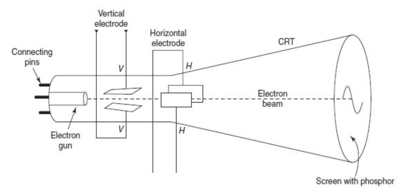
Figure 14-2 Components of a cathode-ray oscilloscope
