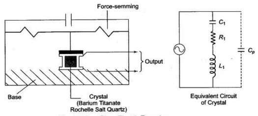
Fig. 13.31 Piezo Electric Transducer
