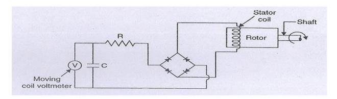
It consists of, like an alternator, a stationary armature (stator) and a rotating field system (rotor). Owing to the generation of e.m.f in a stationary coil on a stator, commutation problems no longer exist. The alternating e.m.f. induced in the stationary coil is rectified, and the output D.C. voltage is measured with the help of a moving coil voltmeter (V).
