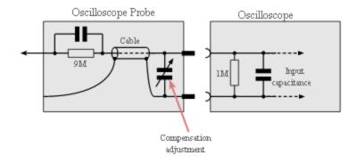
Oscilloscope probe circuit
