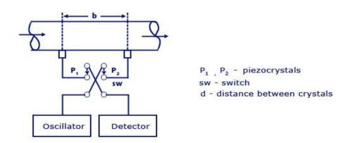
When pressure waves are released into the flowing fluid, their velocity and amplitude are affected by the fluid velocity. Ultrasonic flow meters help in measuring these pressure wave changes, especially in the ones having frequencies greater than 20KiloHertz using specialized techniques. There are two types of ultrasonic flow meters.
