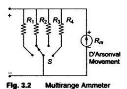
The circuit has four shunts R1,R2,R3 and R4, which can be placed in parallel with the movement to give four different current ranges. Switch S is a multiposition switch, (having low contact resistance and high current carrying capacity, since its contacts are in series with low resistance shunts). Make before break type switch is used for range changing. This switch protects the meter movement from being damaged without a shunt during range changing.
