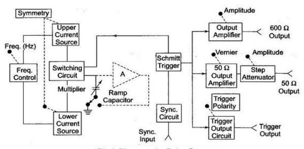
Fig. Block Diagram of a Pulse Generator
