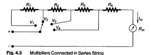
The R1, R2, R3 and R4 are the four series multipliers. When connected in series with the meter, they can give four different voltage ranges as V1, V2, V3, and V4. The selector switch S is multiposition switch by which the required multiplier can be selected in the circuit.
