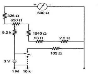
Fig. 4.38 Ohmmeter Section of a Multimeter
