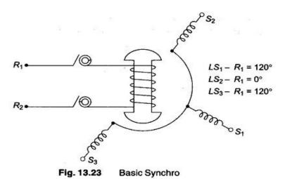
The rotor is energized by an ac voltage and coupling between rotor and stator windings varies as a trigonometric or linear function of the rotor position.
