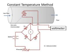
Due to the gas flow, heat transfer takes place from the sensing wire to the flowing gas and this tends to change the temperature and hence the resistance of the wire.
