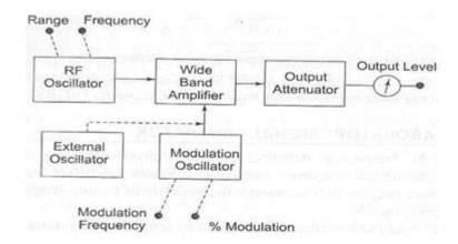
The instrument generates a frequency ranging from 10 Hz to 1 MHz continuously vV (rms). The output is taker through a push-pull amplifier. For low output, the impedance is 6000. The square wave amplitudes can be varied from 0 - 20 v (peak). It is possible to adjust the symmetry of the square wave from 30 -70%. The instrument requires only 7W of power at 220V 50Hz.
