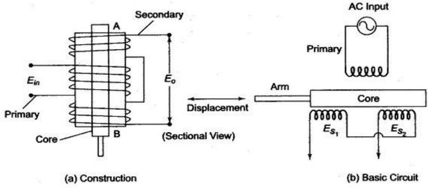
Fig. 13.20 Secondary Winding Connected for Differential Output
