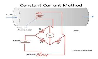
A constant current is passed through the sensing wire. That is, the voltage across the bridge circuit is kept constant, that is, not varied.
