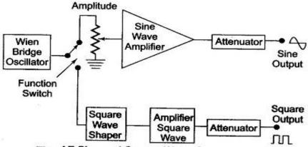
Fig. AF Sine and Square Wave Generator
