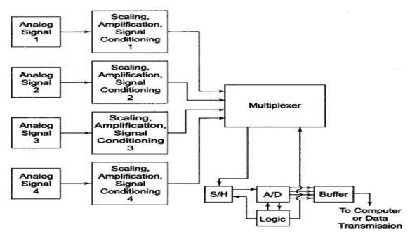
Fig. 17.5 Multi-channel DAS (A/D Preceded by a Multiplexer)
