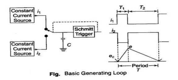
The upper current source supplies a constant current to the capacitor and the capacitor voltage increases linearly. When the positive slope of the ramp voltage reaches the upper limit set by the internal circuit components, the Schmitt trigger changes state. The trigger circuit output becomes negative and reverses the condition of the current switch. The capacitor discharges linearly, controlled by the lower currentsource.
