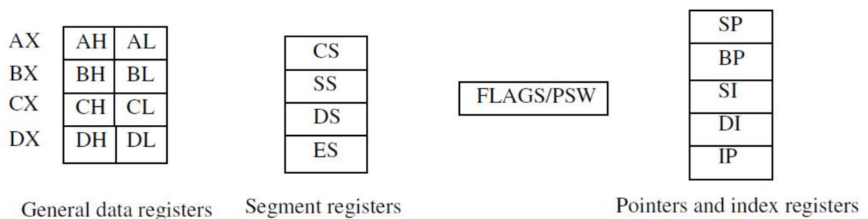
Fig.1.4 Register organization of 8086 Microprocessor
