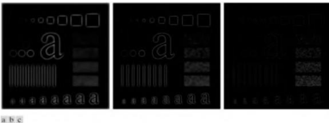
Fig. Results of high-pass filtering the image in fig.(a) using a GHPF with D_0 = 30, 60 and 160 , corresponding to the circles in Fig.(b).
