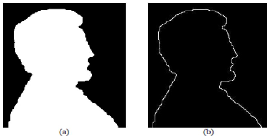
Figure 12.2 (a) Binary image. (b) Object boundary extracted using the previous equation and 3 \times 3 square structuring element.
