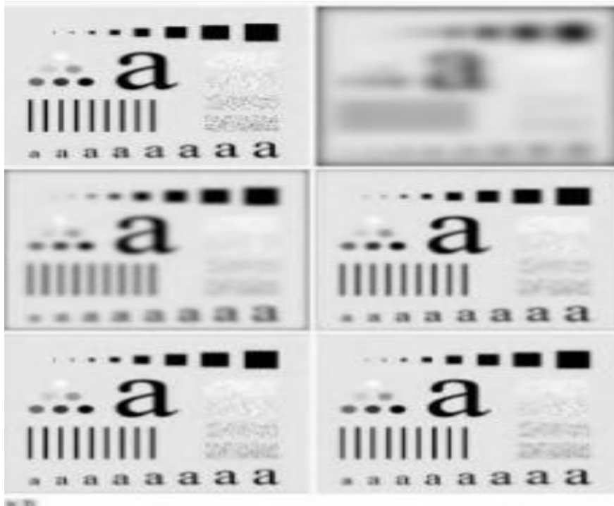
Fig.(a) Original image. (b)-(f) Results of filtering using GLPFs with cutoff frequencies at the radii shown in figure.
