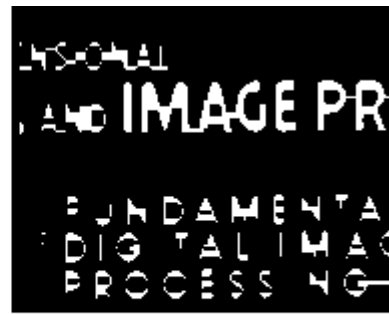
Hit and miss transform: an elongated 2×5 structuring element
