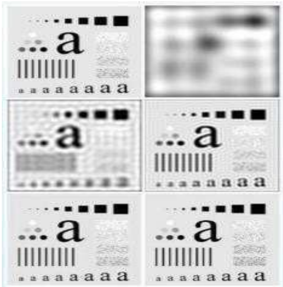
Fig: (a) original image, (b)-(f) Results of filtering using ILPFs with cutoff frequencies set at radii values 10, 30, 60, 160 and 460, as shown in fig.2.2.2(b). The power removed by these filters was 13, 6.9, 4.3, 2.2 and 0.8% of the total, respectively.
