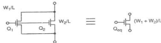
Figure 4.12 Two transistors in parallel ( Q_1 and Q_2 ) having equal L s, are equivalent to a single transistor having a width equal to the sum of the widths of Q_1 and Q_2 .
