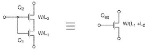
Figure 4.13 Two transistors ( Q_1 and Q_2 ), having equal W s and connected in series, with their gates connected together are equivalent to a single transistor having a length equal to the sum of the lengths of Q_1 and Q_2 .
