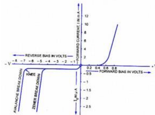
Fig 1.18: Diode characteristics with breakdown
