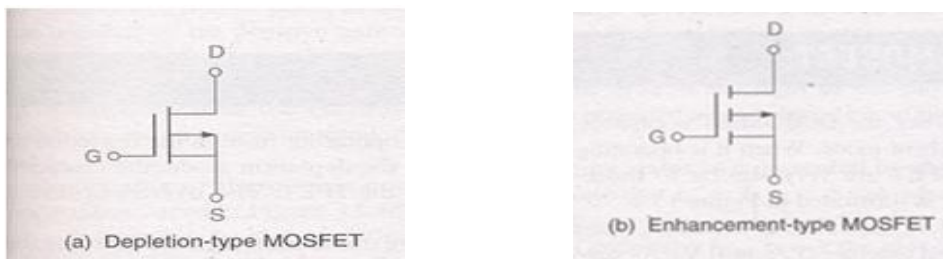
Fig 4.7(a) Depletion type MOSFET (b) Enhancement type MOSFET
