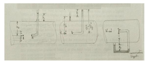
Simplest form of a pitot tube consists of a glass tube, large enough for capillary effects to be negligible and bent at right angles. A single tube of this type is used for measuring the velocity of flow in an open channel. The tube is dipped vertically in the flowing stream of fluid with its open end A directed to face the flow and other open end projecting above the fluid surface in the stream. The fluid enters the tube and the level of the Department of Mechanical Engineering, MRCET
