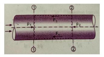
Consider a uniform horizontal pipe having steady flow. Let 1-1, 2-2 are two sections of pipe.
