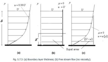
Fig. 5.7.3: (a) Boundary layer thickness; (b) Free stream flow (no viscosity) (c) Concepts of displacement thickness.
