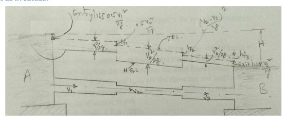
If a pipe line connecting two reservoirs is made up of several pipes of different diameters d<sub>1</sub>, d<sub>2</sub>, d<sub>3</sub>, etc. and lengths L<sub>1</sub>, L<sub>2</sub>, L<sub>3</sub> etc. all connected in series (i.e. end to end), then the difference in the liquid surface levels is equal to the sum of the head losses in all the sections. Further the discharge through each pipe will be same.
