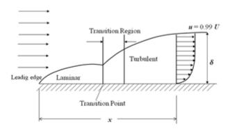
Fig. 1: Representation of boundary layer on a flat plate.
