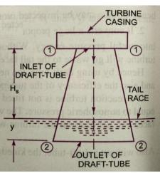
$$\frac{p_{1}}{\rho g} = \frac{p_{a}}{\rho g} + \frac{{V_{2}}^{2}}{2g} + h_{f} - \frac{{V_{1}}^{2}}{2g} - H_{s}$$
