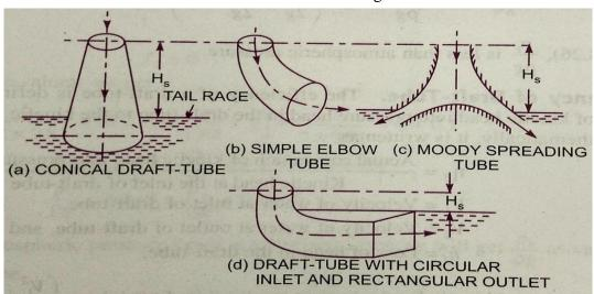
and moody spreading draft tubes are most efficient while simple elbow draft tube and elbow draft tubes with circular inlet and rectangular outlet require less space as compared to other draft tubes.
