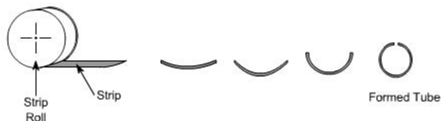
Fig 11.10: Forming of Tube from Strip
