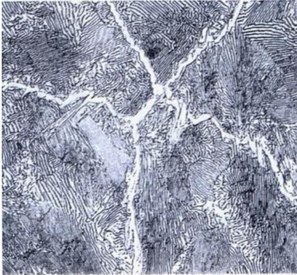
Hypo-eutectoid steel showing primary cementite along grain boundaries pearlite
