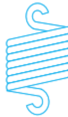
(b) Tension helical spring.
