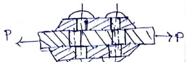
Fig: Double shear (b) of a riveted joint.
