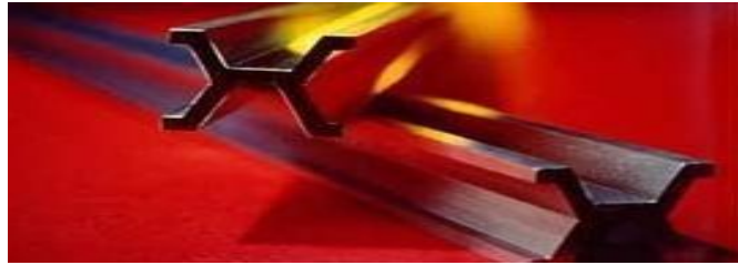
Historical International Prototype Meter bar, made of an alloy of platinum and iridium, that was the standard from 1889 to 1960.
