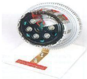
Fig: Cutaway Model Of Multi-Plate Clutch
