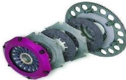
Fig: Exploded View Of Multi-Plate Clutch
