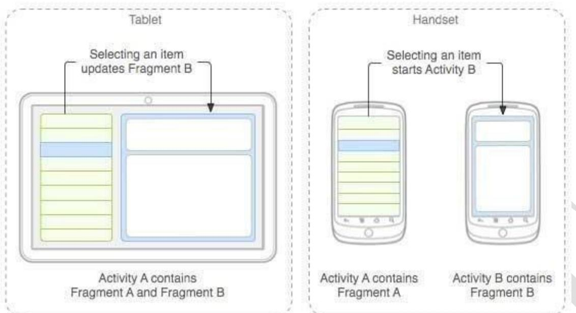
The application can embed two fragments in Activity A, when running on a tablet-sized device. However, on a handset-sized screen, there's not enough room for both fragments, so Activity A includes only the fragment for the list of articles, and when the user selects an article, it starts Activity B, which includes the second fragment to read the article.
