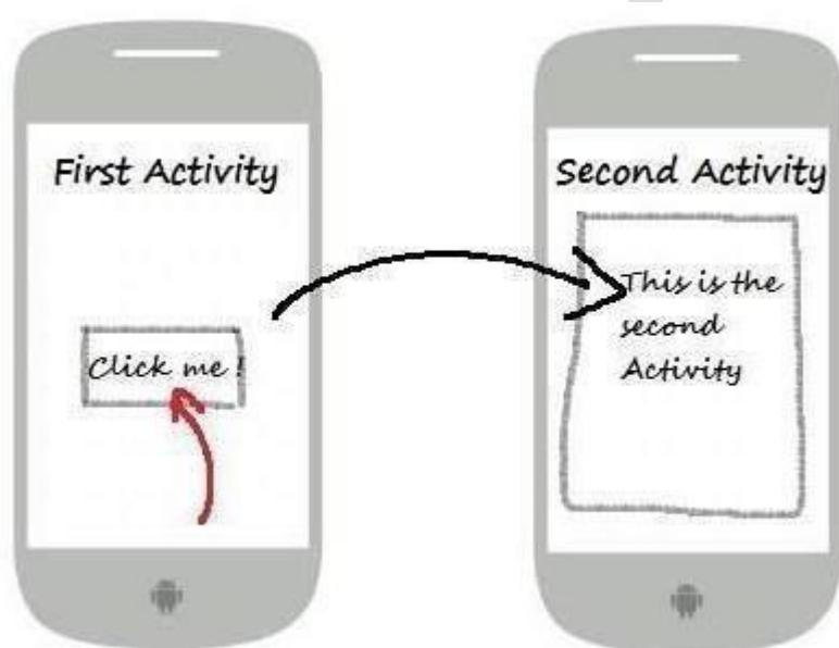
These intents designate the target component by its name and they are typically used for application-internal messages - such as an activity starting a subordinate service or launching a sister activity. For example –
