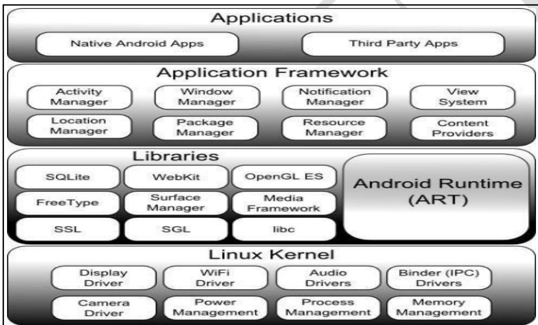
Android is structured in the form of a software stack comprising applications, an operating system, run-time environment, middleware, services and libraries. Each layer of the stack, and the corresponding elements within each layer, are tightly integrated and carefully tuned to provide the optimal application development and execution environment for mobile devices.
