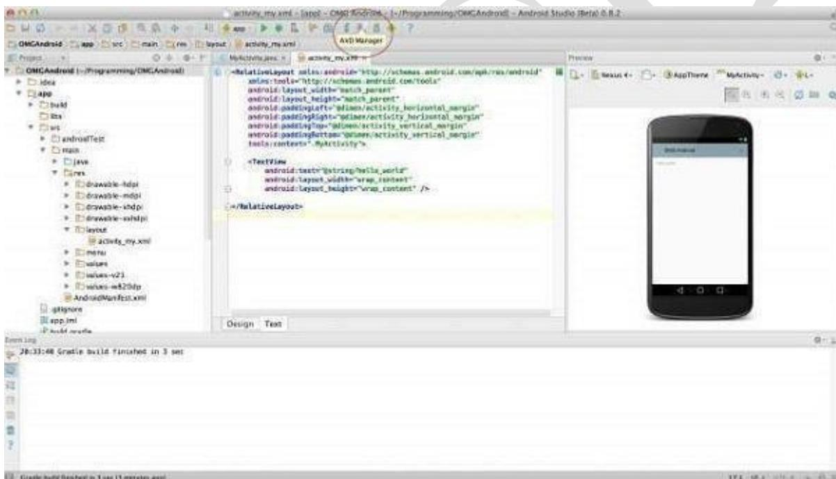
After Click on a virtual device icon, it going to be shown by default virtual devices which are present on your SDK, or else need to create a virtual device by clicking **Create new Virtual device** button
