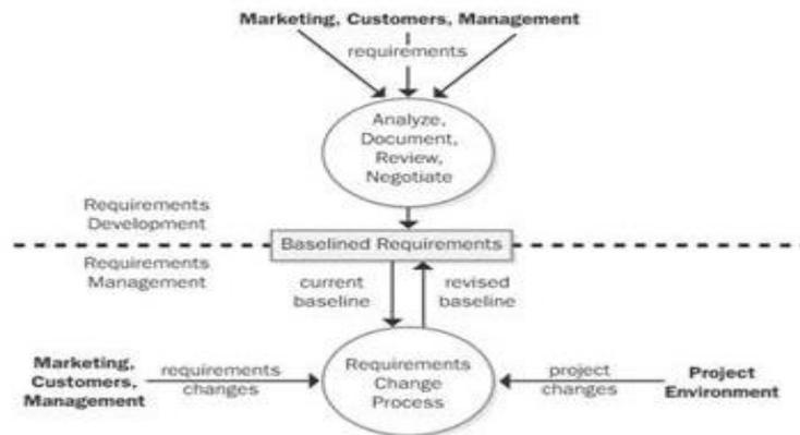
**Figure 1-3:** The boundary between requirements development and requirements management.
