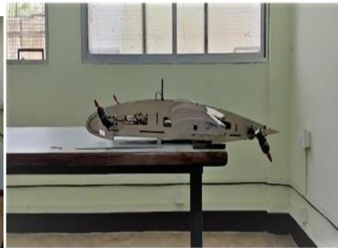
Bench test of tilt rotor mechanism at full throttle
